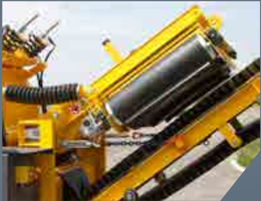
Magnetic Separator Rebar and wire removal with on-board permanent magnet.
