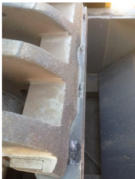
The picture shows a worn rotor body. The previous operator didn't change the hammers in time.
