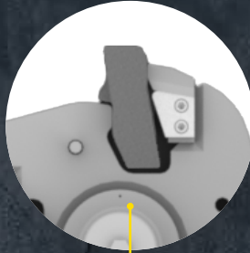
HALF WORN HAMMER needs to be flipped
