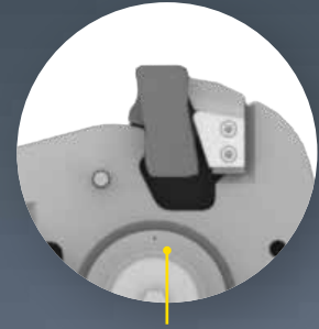
FULLY WORN HAMMER needs to be changed (or kept as short hammers)
