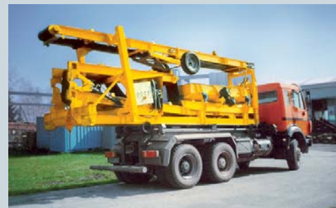
Compact, lightweight and mobile: the CS2500 is quickly transported to any job site using a hook-lift truck
