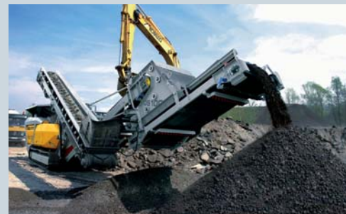
Unrestricted mobility on-site for RM crusher mounted on crawler gear plus oversized grain system
