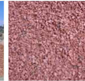
Recycled brick chippings
