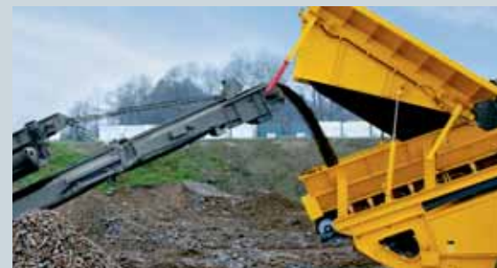
The TS3600 can be fed either by a wheel loader or directly by a RUBBLE MASTER crusher.
