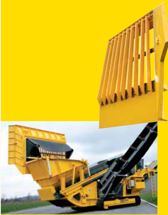
Oversize grain mesh of the feed hopper can be tilted 90° using remote control
