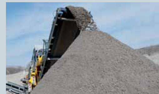
The long, hydraulic fold-in discharge belts can be adjusted steplessly up to 13' discharge height.
