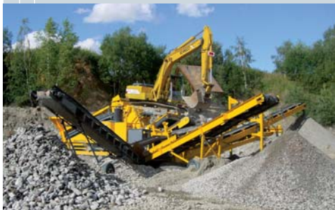
Maintain a production rate of up to 112 tons/h (100 tonnes/hr) with the double-deck version while achieving the highest separation accuracy
